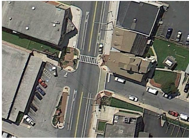
Aerial view of Harford Road curb extensions with clearly delineated crosswalks, landscaping and improved pedestrian safety.
